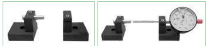
Controllo comparatori. Control of dial gauges.
